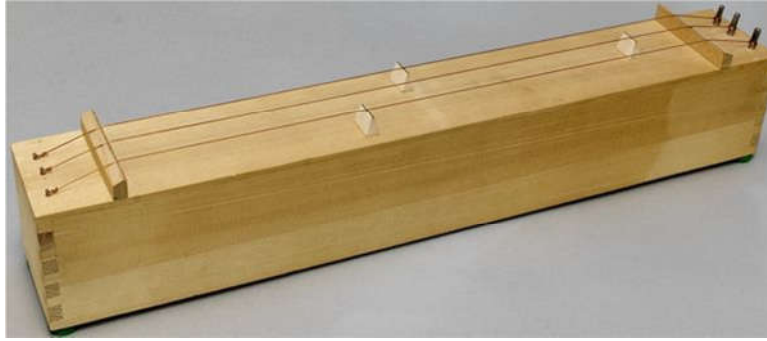
Figure 16: Monochord and its proportions.
